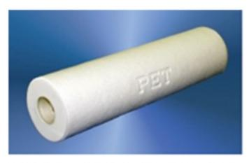
PET Melt Blown depth filter cartridges are designed for applications where use of polypropylene or Nylon is limited due to high temperature or compatibility issues. These cartridges also offer true gradient depth filtration, with extremely low pressure drops and high void volumes to ensure long service life of the filter.
